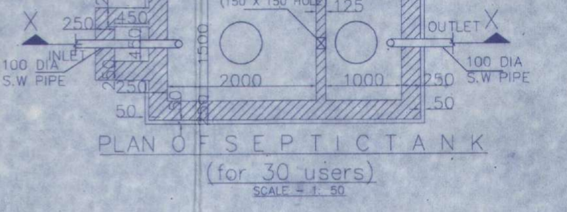
PLAN OF SEPTICTANK (for 30 users) SCALE - 1:50
